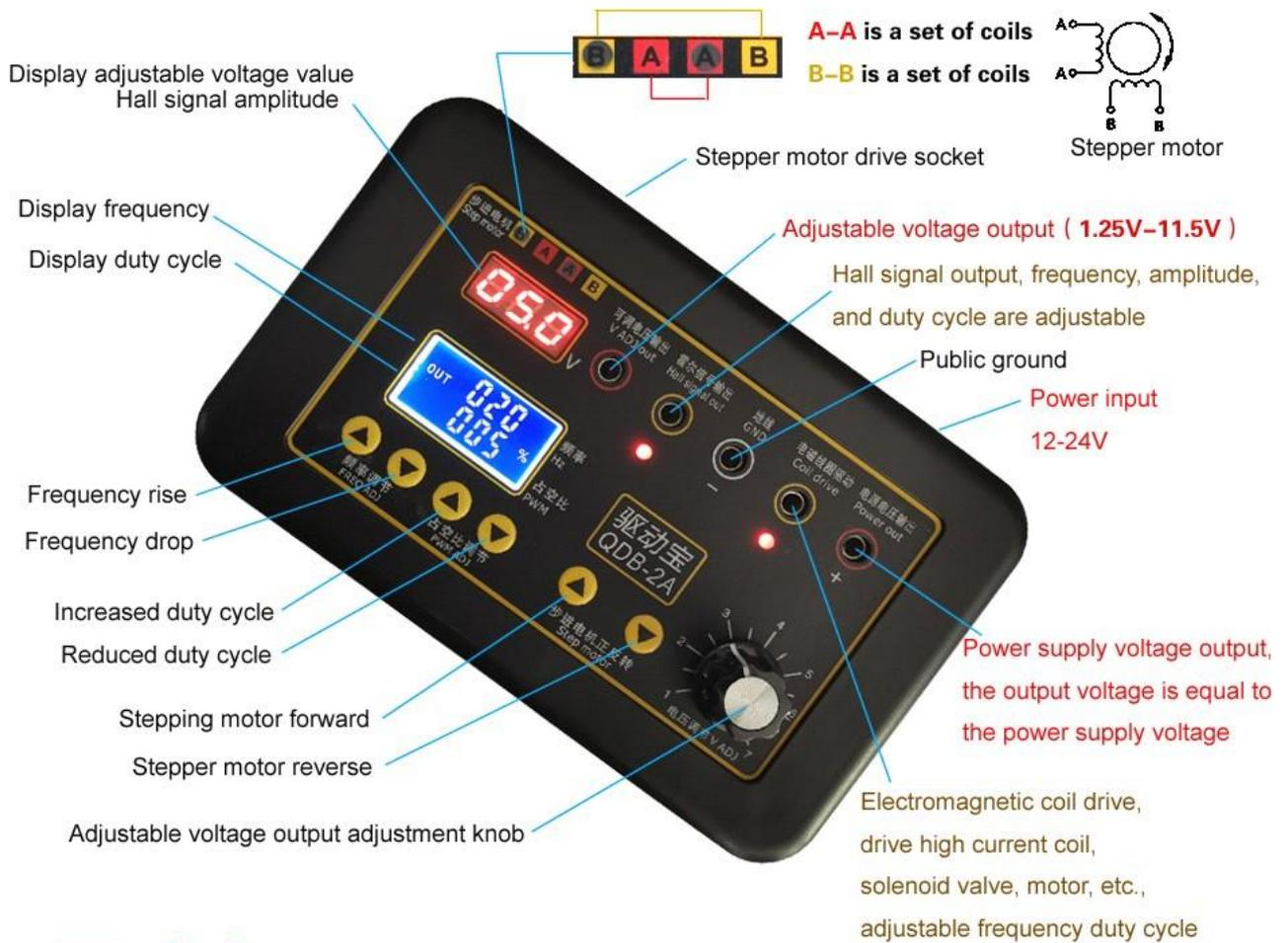
**驱动宝 QDB-2A** Automobile actuator drive detector
